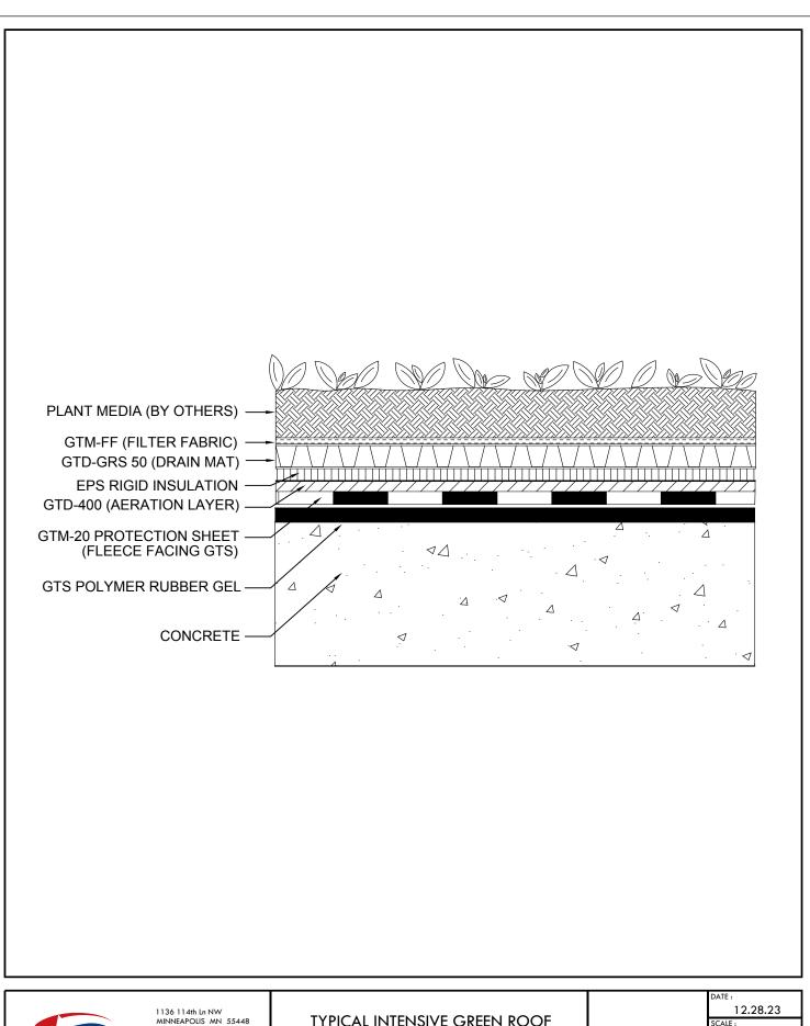
OFFICE: 612. 872. 1900 www.re-systemsgroup.com TYPICAL INTENSIVE GREEN ROOF DETAIL
